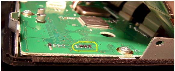
Remove D53, D54 and D55. Reset of the radio will probably not be necessary. Reassemble radio and test.
